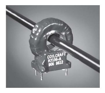
The CS60 series is designed tomeasure current from 5 to 100 Arms. Applications include sensing branch circuit overload and detecting load drop or shutdown. The sensor functions as the encapsulated secondary of a current transformer, while the conductor carrying the current to be measured serves as the "one turn primary." Sensitivity may be enhanced by increasing primary turns.
